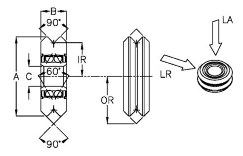
$\begin{array}{ll} \mbox{Diameter A} & = 75.39 \\ \mbox{Hole size C} & = 22.00 \\ \mbox{Internal radius IR} = 31.75 \\ \mbox{Outer radius OR} & = 44.45 \\ \mbox{Width B} & = 25.40 \\ \end{array}$
